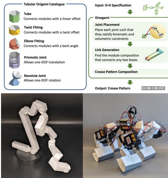
Fig. 5: Modular approach to origami mechanism design. Bottom: Example 6-degree-of-freedom chain and quadrupedal robot generated using the algorithm in [3].
